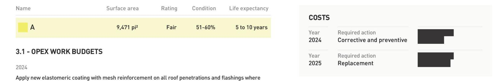
required to eliminate water ingression. Adequately seal and secure the existing metal perimeter flashings back into position.
